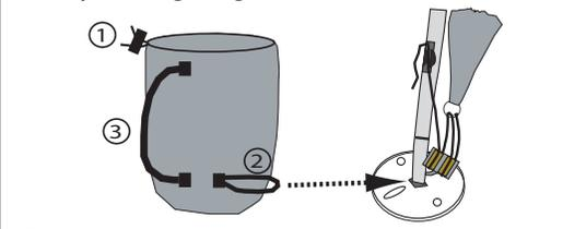
① Fill the weight-bag inlet with water/sand/stones/snow etc. and close the bag with the cord on the upper side of the bag. ①
