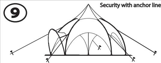
thread the anchor lines (fixed on the tunnels) as wide as possible away from the dome and drive the stakes into the ground. Then fix the rope at the upper part of the stake. Furthermore drive the stakes through the hole at each footpad to fix the legs and secure the dome.
