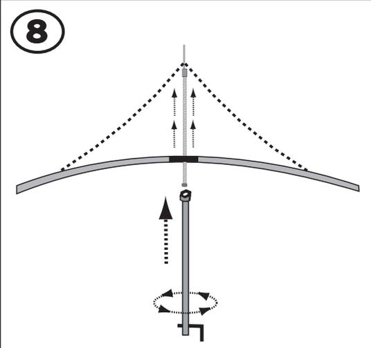
hold the cupola wrench to the bottom part of the cupola shaft and turn the wrench to raise the cupola until fabric becomes wrinkle free. Caution: do not over tighten !!
