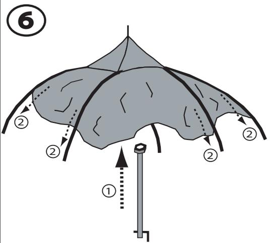
one person is going under the fabric and raise the Dome with the cupola wrench. ①
