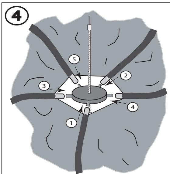
place the cupola hub with the fixed cupola shaft into the center opening of the fabric. (the long part of the shaft on upper side). Then connect the frame legs to the cupola hub. Please mind to do this according to No. 1 - 5. Sliding the fabric inward towards the center opening will ease the legs connection to the hub.
